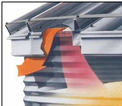
Unique Eave-Vent System raises the roof off the sidewalls to create ample ventilation around the entire circumference of the bin. The result is more air circulation while eliminating roof cuts, all at a lower cost than rooftop ventilation options.
