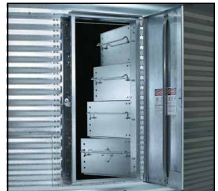
LATCH-LOCK® Walk-Through Bin Entry Doors offer simple yet safe access, with a one-piece outer door and four interlocking inner panels that open in sequence from top to bottom with a lift of a latch.
