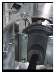
**Totally-enclosed C-face motor** is mounted directly to an in-line gear reducer for no loss of horsepower and no belts to maintain or replace.
