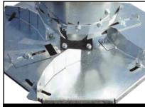
**Spreader impellers** can be adjusted to match the grain throw distance to the bin's diameter.
