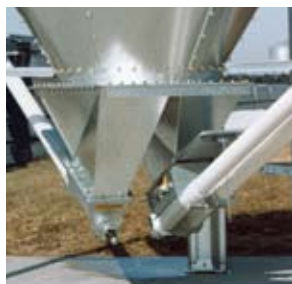
B - Boot with three auger systems servicing two buildings (Model 75 FLEX-AUGER® shown.)
